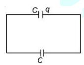
$$V_c = \frac{q_1 + q_2}{C_1 + C_2} = \frac{q + 0}{C + C}$$
