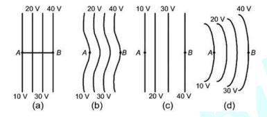
A positive charge is moved from A to B in each diagram.
